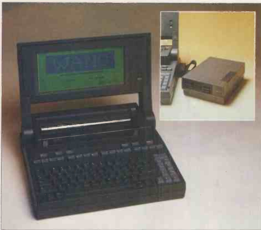
Hard disc and printer (below) are built in, but to load from a floppy you need an external drive (inset).
